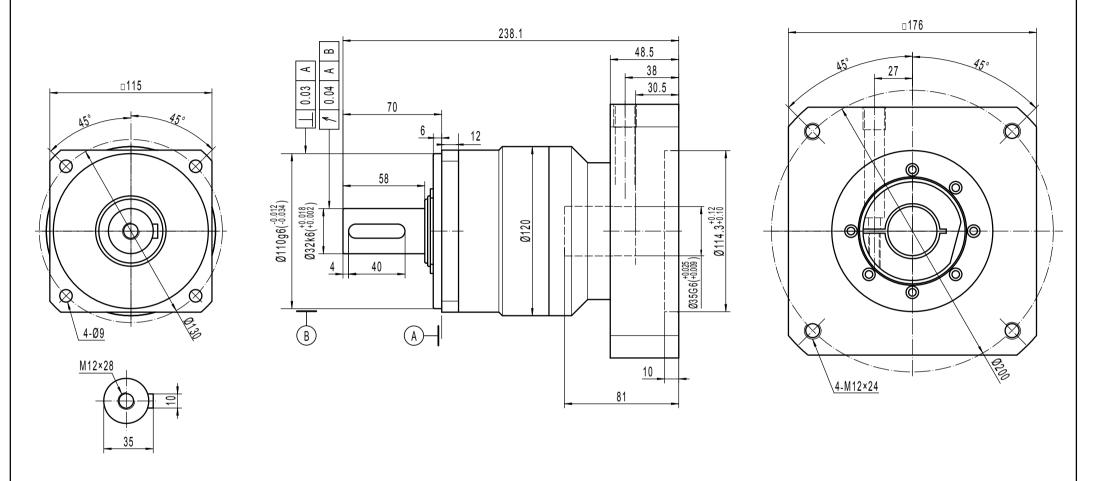
Note 1: This drawing shows the dimensions of ACCESS-SQ-ST-120 - 1 STAGE (this drawing is common to ratios 3 to 10)
