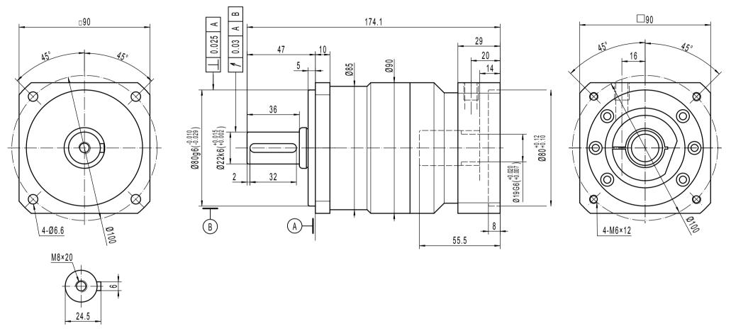
Note 1: This drawing shows the dimensions of ACCESS-SQ-ST-090 - 1 STAGE (this drawing is common to ratios 3 to 10)
