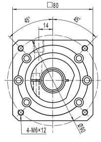
Note 1: This drawing shows the dimensions of ACCESS-SQ-ST-090 - 1 STAGE (this drawing is common to ratios 3 to 10)
