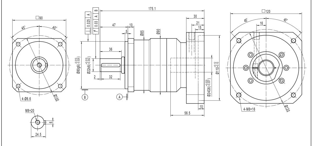
Note 1: This drawing shows the dimensions of ACCESS-SQ-ST-090 - 1 STAGE (this drawing is common to ratios 3 to 10)
