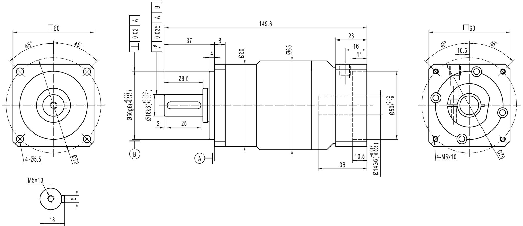
Note 1: This drawing shows the dimensions of ACCESS-SQ-ST-060 - 2 stages (It is common to all ratios from 12 to 100)
