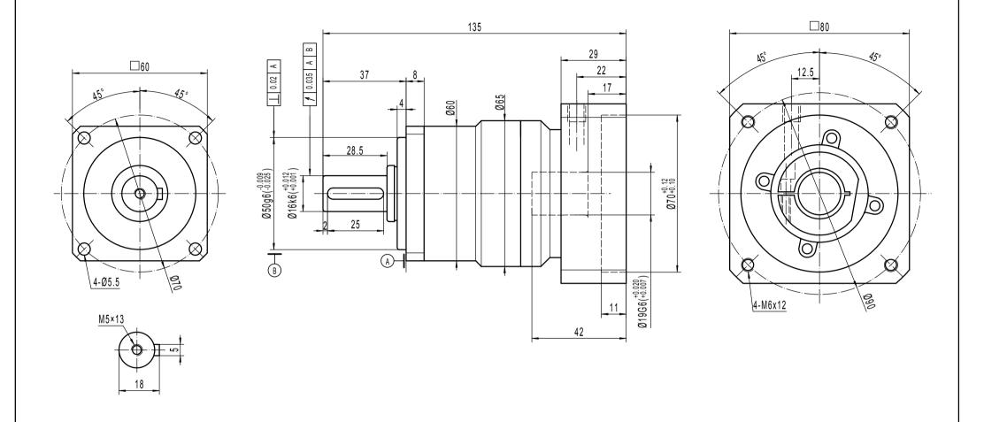
Note 1: This drawing shows the dimensions of ACCESS-SQ-ST-060- 1 STAGE (this drawing is common to ratios 3 to 10)
