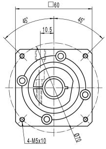
Note 1: This drawing shows the dimensions of ACCESS-SQ-ST-060 - 1 STAGE (this drawing is common to ratios 3 to 10)
