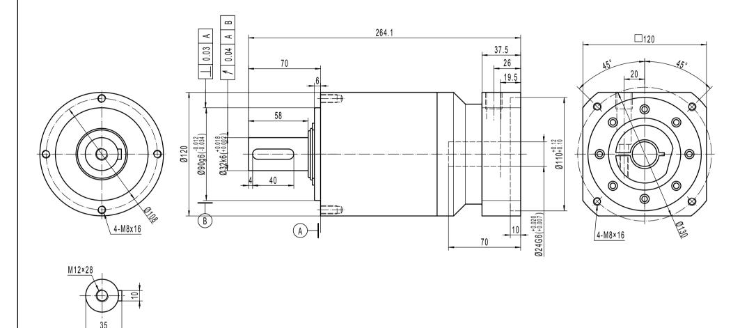
Note 1: This drawing shows the dimensions of ACCESS-CI-ST-120 - 2 STAGES (drawing common to ratios 12 to 100)
