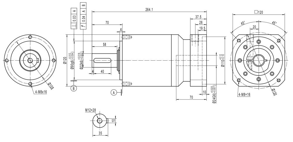
Note 1: This drawing shows the dimensions of ACCESS-CI-ST-020 - 2 STAGES (drawing common to ratios 12 to 100)
