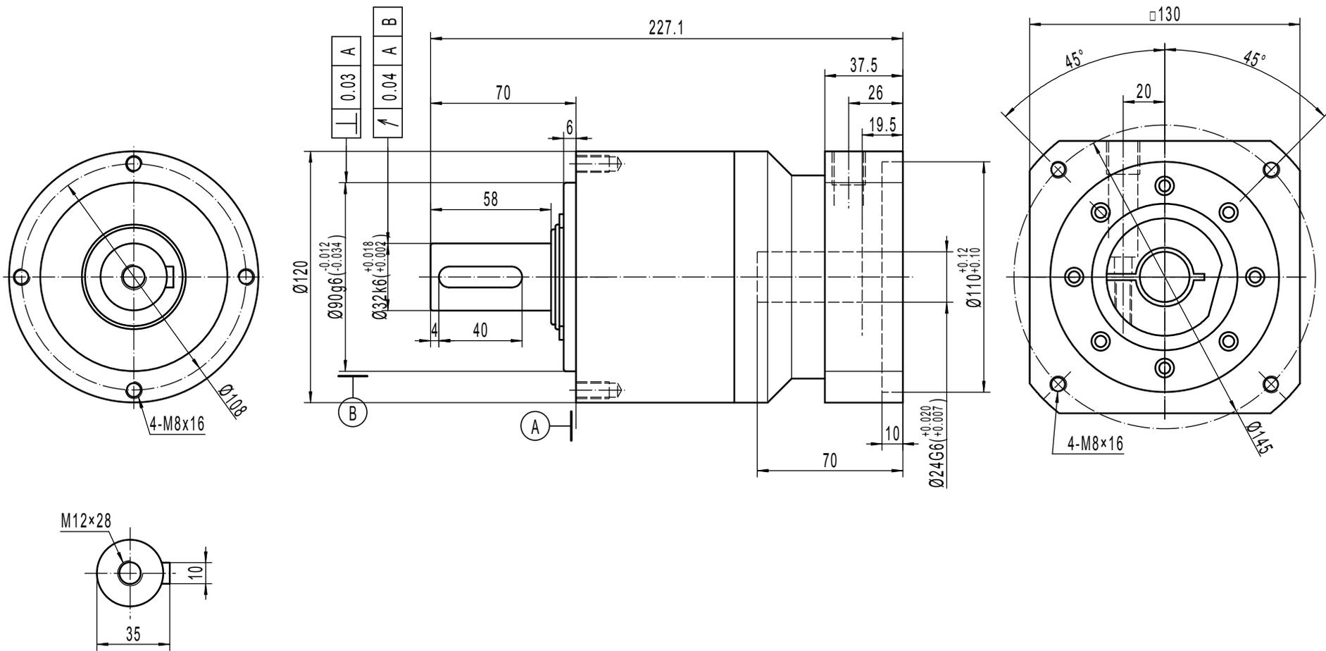
Note 1: This drawing shows the dimensions of ACCESS-CI-ST-120 - 1 STAGE (drawing common to ratios 3 to 10)
