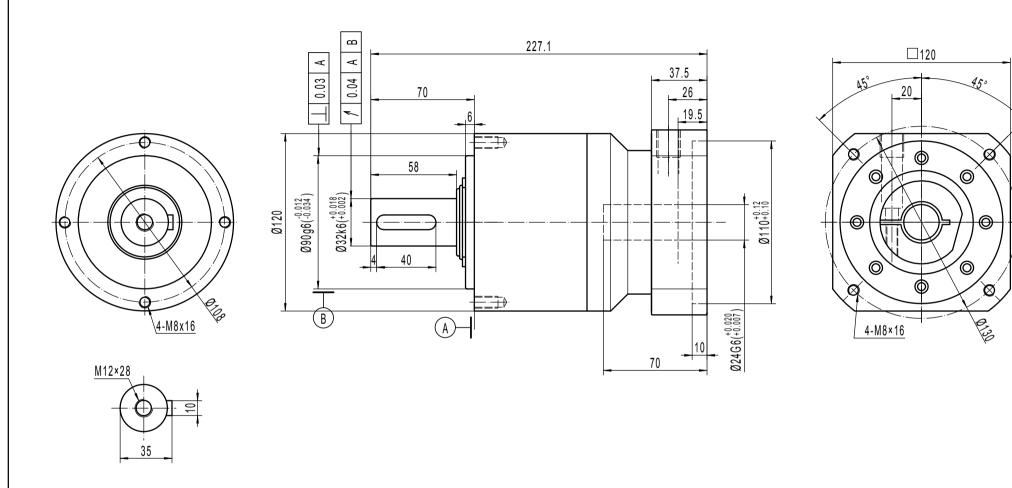
Note 1: This drawing shows the dimensions of ACCESS - CI - ST - 120 1 STAGE (this drawing is common to ratios 3 to 10)
