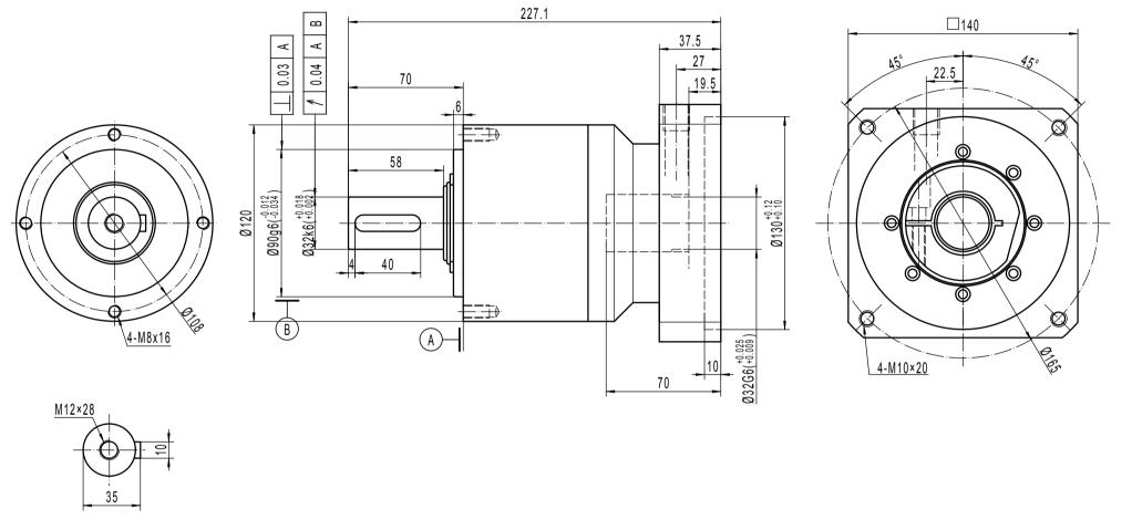
Note 1: This drawing shows the dimensions of ACCESS-CI-ST-120 - 1 STAGE (drawing common to ratios 3 to 10)
