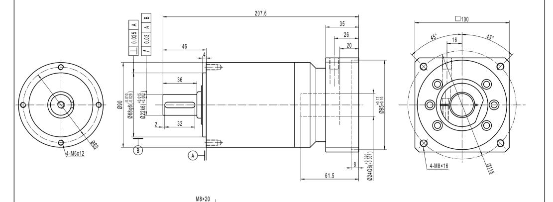
Note 1: This drawing shows the dimensions of ACCESS-CI-ST-090 - 2 STAGES (drawing common to ratios 12 to 100)
