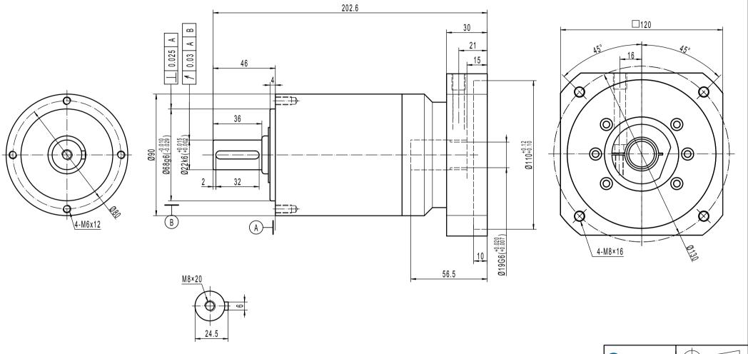
Note 1: This drawing shows the dimensions of ACCESS-CI-ST-090 - 2 STAGES (drawing common to ratios 12 to 100)
