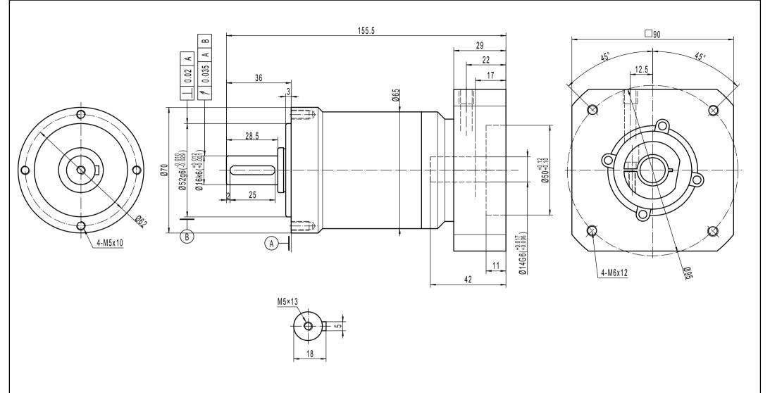
Note 1: This drawing shows the dimensions of ACCESS-CI-ST-070 - 2 STAGES (drawing common to ratios 12 to 100)
