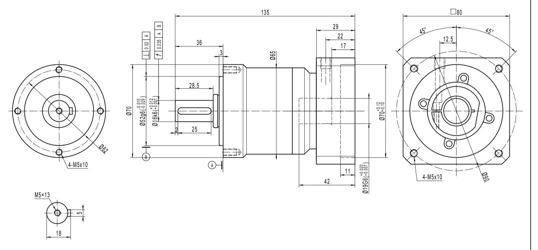
Note 1: This drawing shows the dimensions of ACCESS-CI-ST-070- 1 STAGES (drawing common to ratios 3 to 10)
