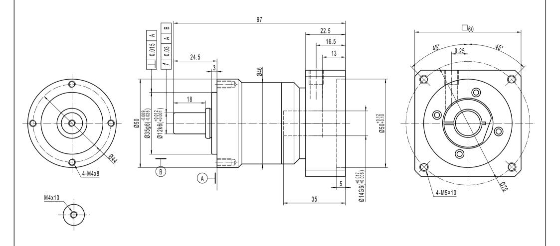
Note 1: This drawing shows the dimensions of ACCESS - CI - ST - 050 – 1 STAGE (this drawing is common to ratios 3 to 10)
