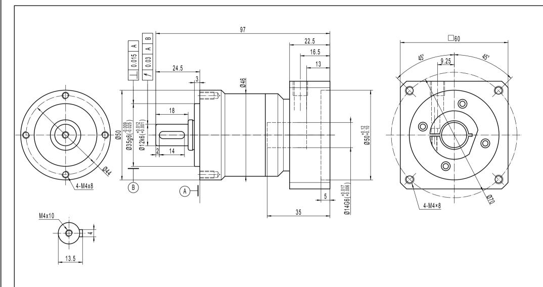
Note 1: This drawing shows the dimensions of ACCESS-CI-ST-050- 1 STAGE (drawing common to ratios 3 to 10)
