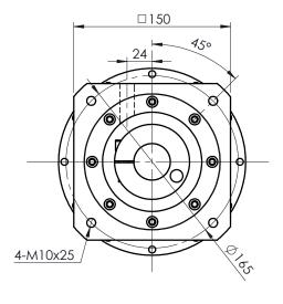
A bushing will be supplied if your motor shaft is smaller than ø35mm
