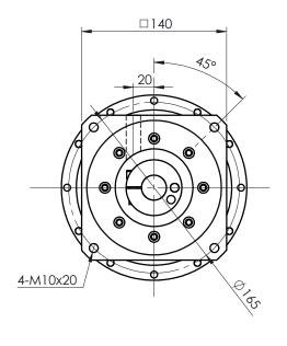
A bushing will be supplied if your motor shaft is smaller than Ø24mm
