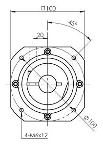
A bushing will be supplied if your motor shaft is smaller than ø24mm
