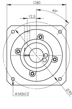
A bushing will be supplied if your motor shaft is smaller than ø19mm
