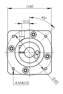
A bushing will be supplied if your motor shaft is smaller than Ø14mm
