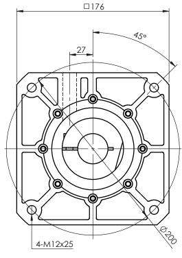
A bushing will be supplied if your motor shaft is smaller than ø35mm
