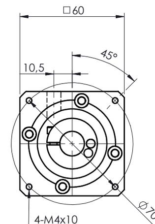
A bushing will be supplied if your motor shaft is smaller than  $\varnothing 14\text{mm}$
