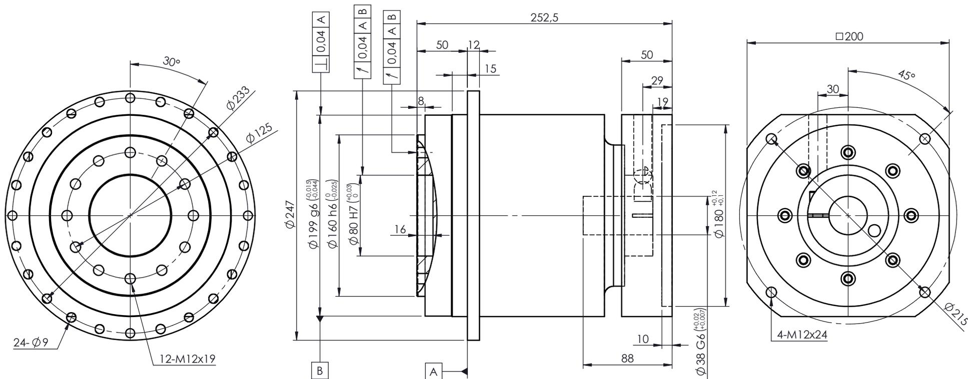
A bushing will be supplied if your motor shaft is smaller than  $\phi 38\text{mm}$
