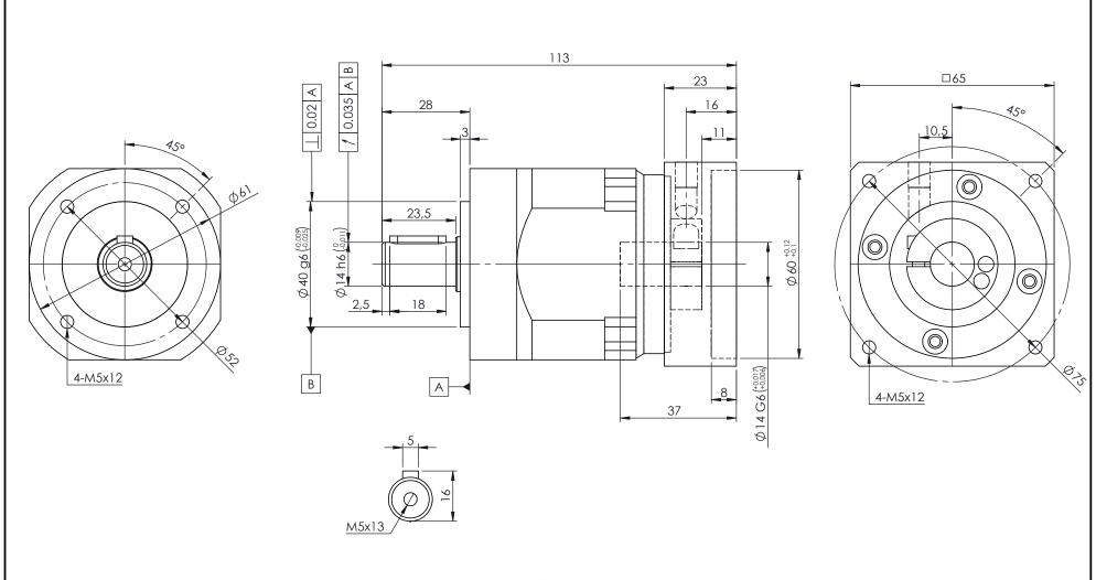
A bushing will be supplied if your motor shaft is smaller than Ø14mm
