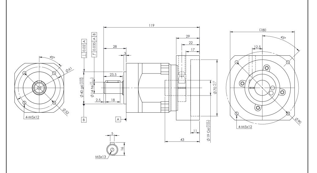
A bushing will be supplied if your motor shaft is smaller than Ø19mm
