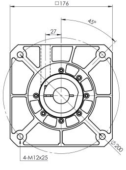
A bushing will be supplied if your motor shaft is smaller than ø28mm
