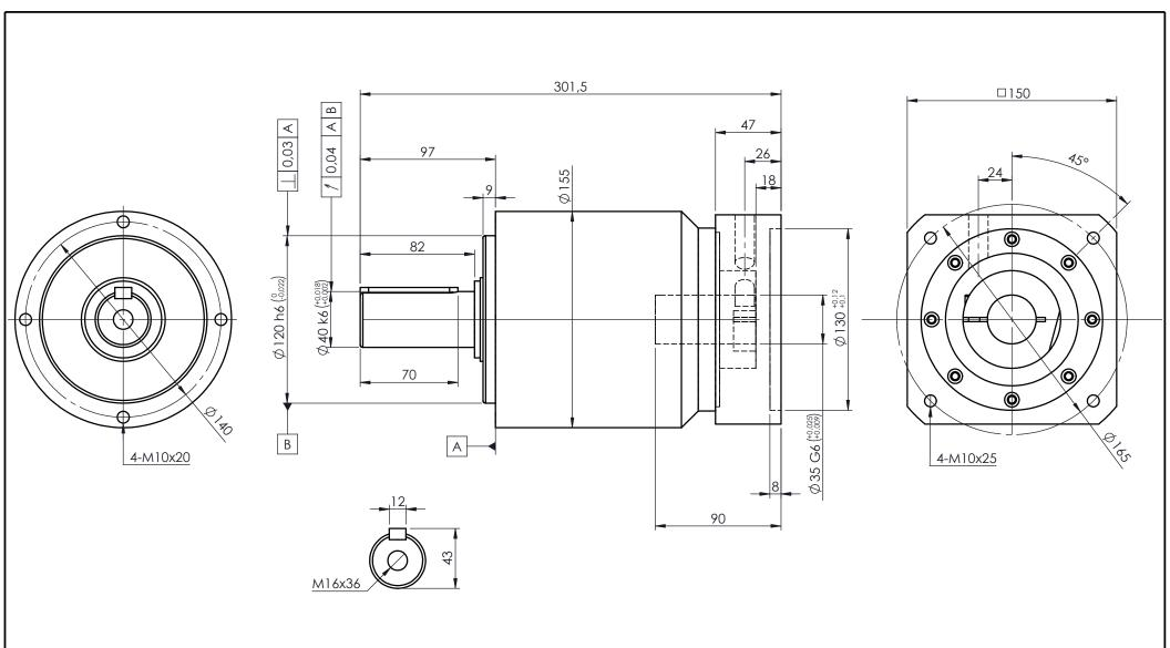
A bushing will be supplied if your motor shaft is smaller than ø35mm
