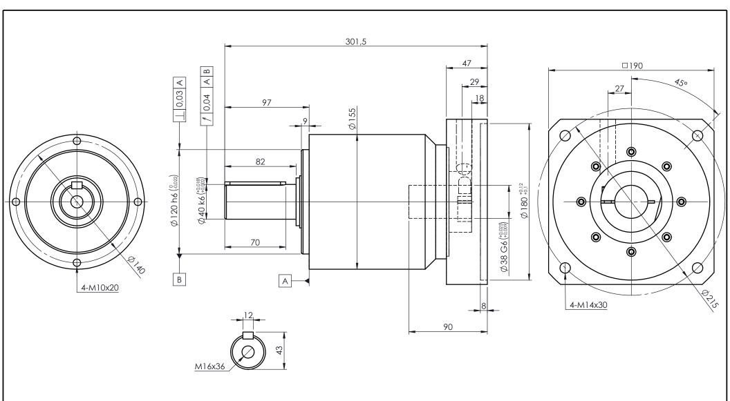
A bushing will be supplied if your motor shaft is smaller than ø38mm
