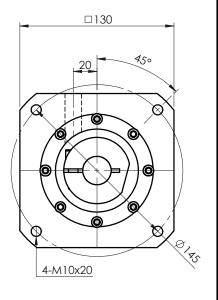
A bushing will be supplied if your motor shaft is smaller than ø24mm
