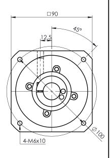
A bushing will be supplied if your motor shaft is smaller than ø19mm
