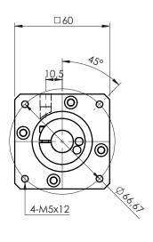
A bushing will be supplied if your motor shaft is smaller than Ø14mm
