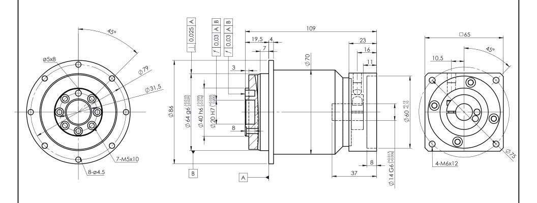
A bushing will be supplied if your motor shaft is smaller than ø14mm
