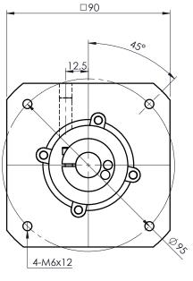
A bushing will be supplied if your motor shaft is smaller than ø14mm
