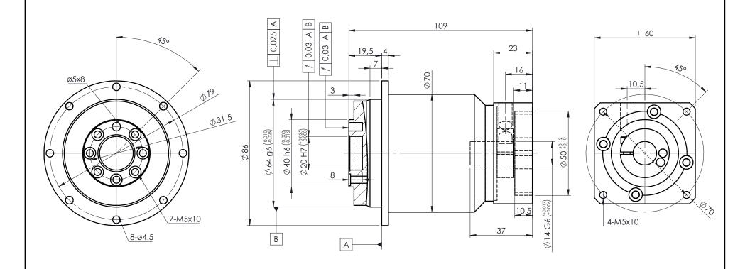
A bushing will be supplied if your motor shaft is smaller than ø14mm
