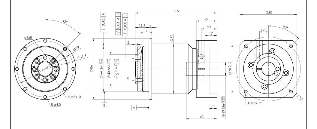
A bushing will be supplied if your motor shaft is smaller than Ø19mm
