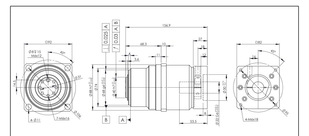
A bushing will be supplied if your motor shaft is smaller than ø22mm
