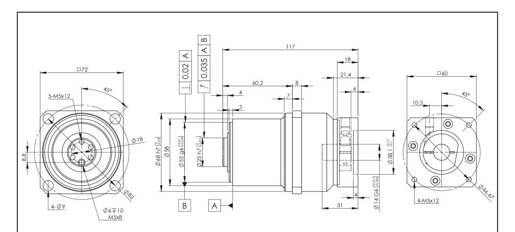
A bushing will be supplied if your motor shaft is smaller than Ø14mm
