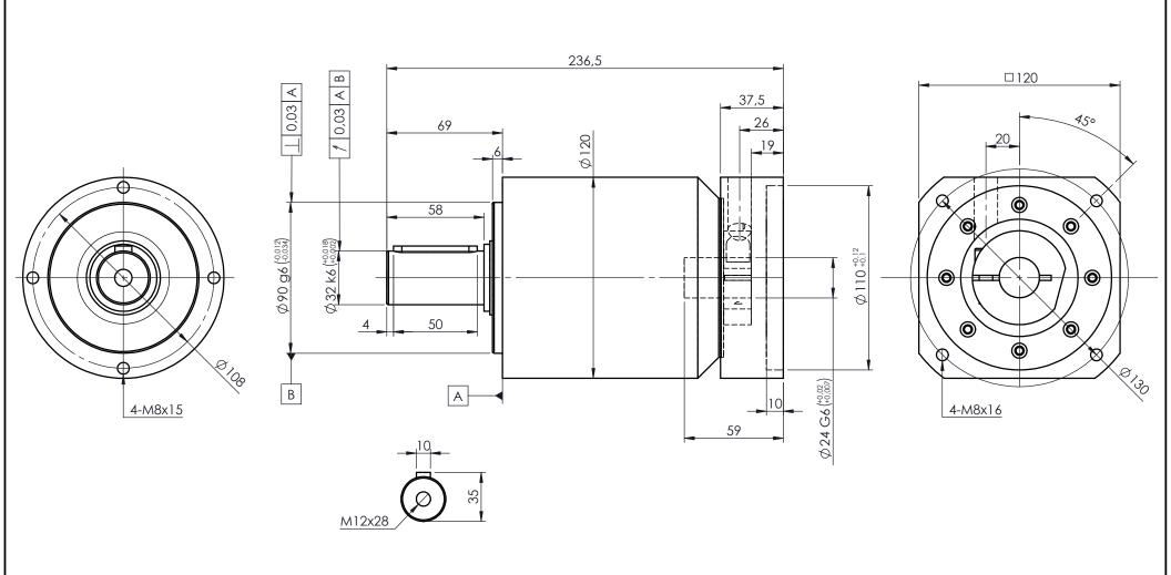
A bushing will be supplied if your motor shaft is smaller than ø24mm
