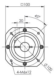
A bushing will be supplied if your motor shaft is smaller than ø24mm
