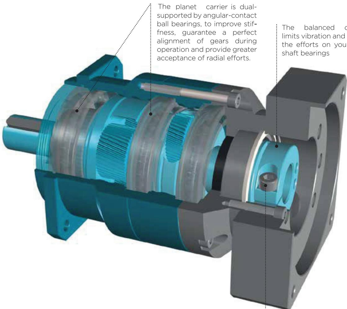
The planet carrier is dual-supported by angular-contact ball bearings, to improve stiffness, guarantee a perfect alignment of gears during operation and provide greater acceptance of radial efforts.
