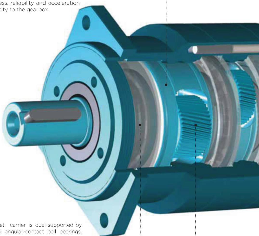
The planet carrier is dual-supported by preloaded angular-contact ball bearings, to improve stiffness, guarantee a perfect alignment of gears during operation and provide greater acceptance of radial efforts.
