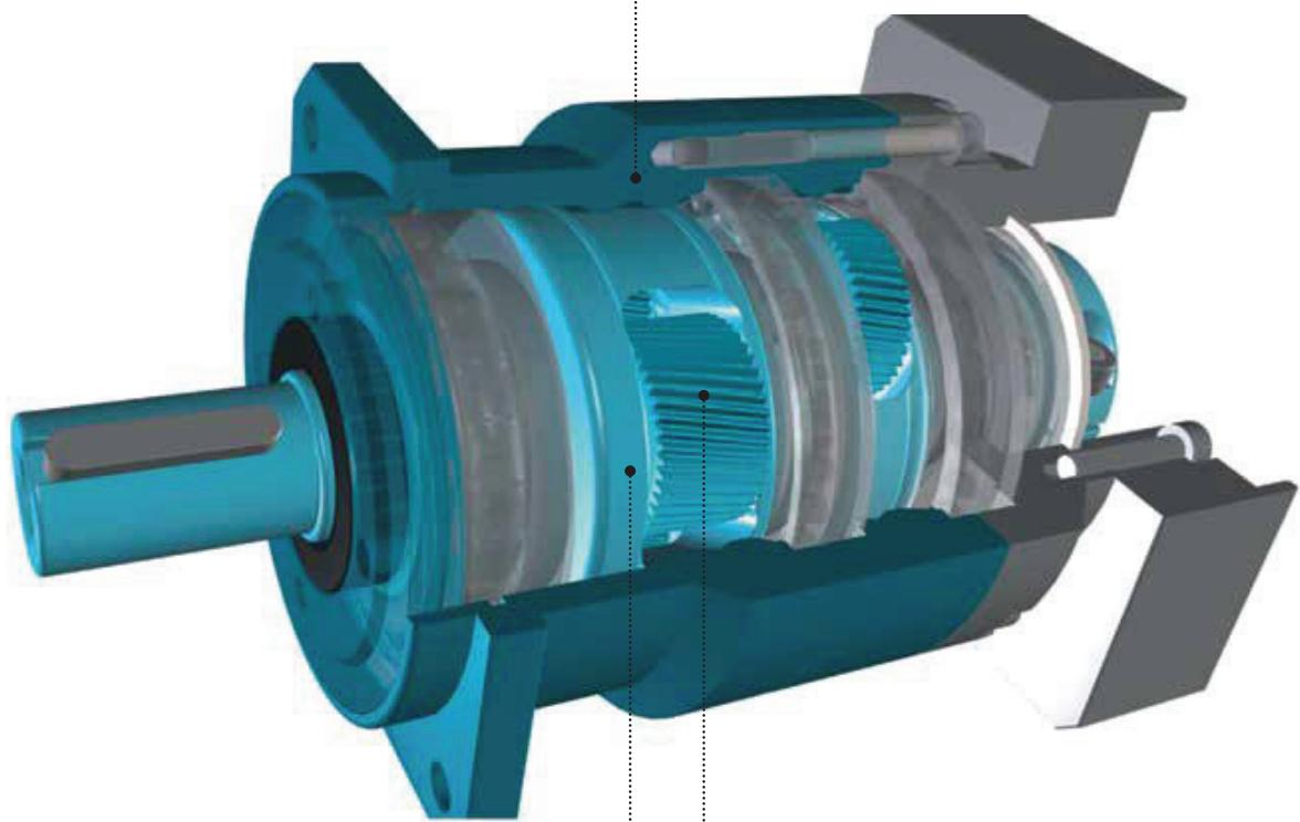
The ring gear is monobloc with the external housing and the output flange, to provide higher stiffness and allow very dynamic reversals.
