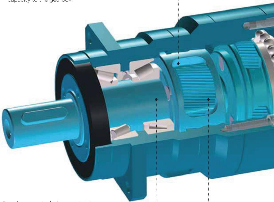
The planet carrier is dual-supported by preloaded tapered roller bearings, to improve stiffness, guarantee a perfect alignment of gears during operation and provide greater acceptance of radial efforts.
