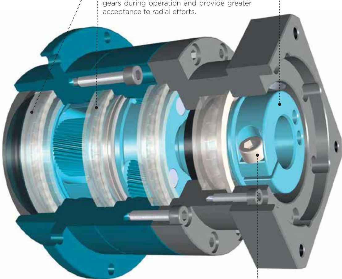
Planet carrier is dual-supported by angular-contact ball bearings (small sizes) or tapered roller bearings (sizes above 140), to improve stiffness, guarantee a perfect alignment of gears during operation and provide greater acceptance to radial efforts.
