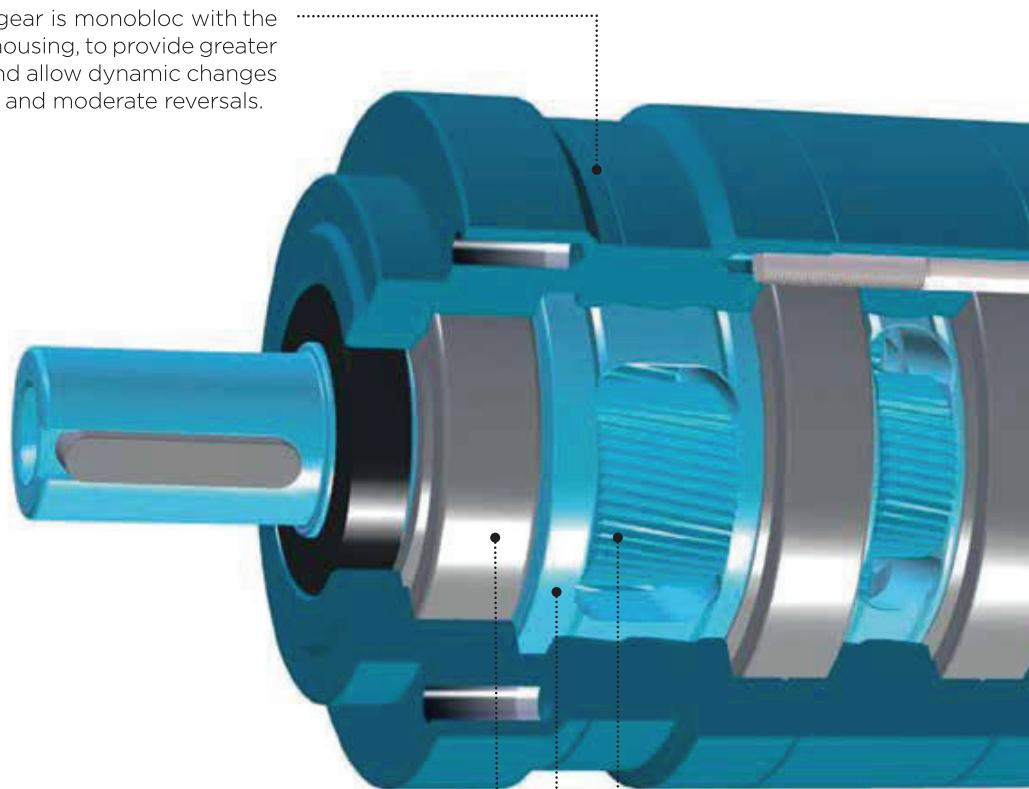
The planet carrier is dual-supported by radial ball bearings, to improve stiffness and guarantee a perfect alignment of gears during operation.
