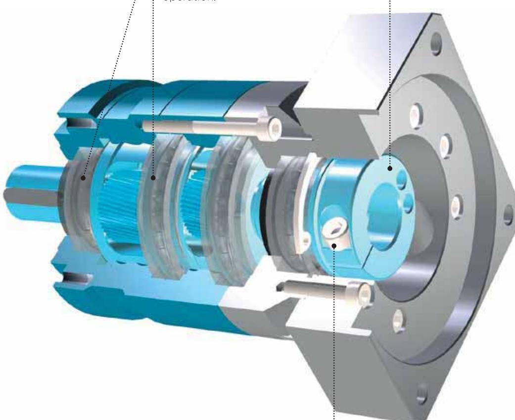
The planet carrier is dual-supported by radial ball bearings. This configuration improves stiffness and thus guarantees the perfect alignment of gears during operation.
