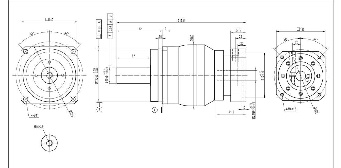
Note 1: This drawing shows the dimensions of X-Treme-SQ-ST-140 - 2 STAGES (this drawing is common to ratios 3 to 10)
