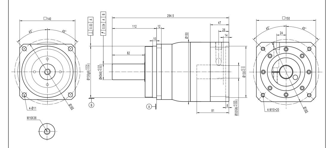
Note 1: This drawing shows the dimensions of X-Treme-SQ-ST-140 - 1 STAGE (this drawing is common to ratios 3 to 10)
