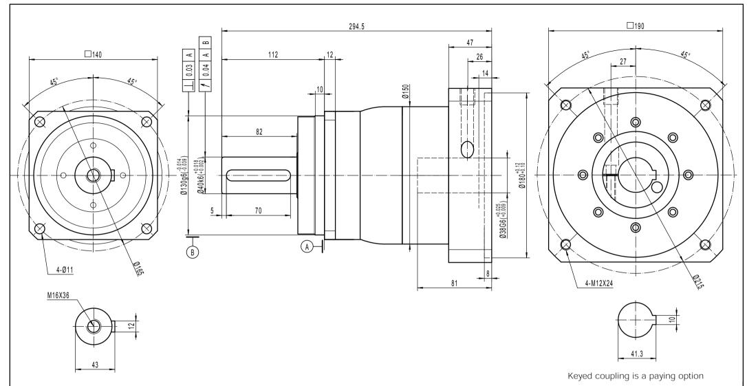
Note 1: This drawing shows the dimensions of X-Treme-SQ-ST-140 - 1 STAGE (this drawing is common to ratios 3 to 10)
