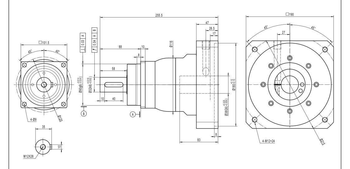
Note 1: This drawing shows the dimensions of X-Treme-SQ-ST-100 - 1 STAGE (this drawing is common to ratios 3 to 10)
