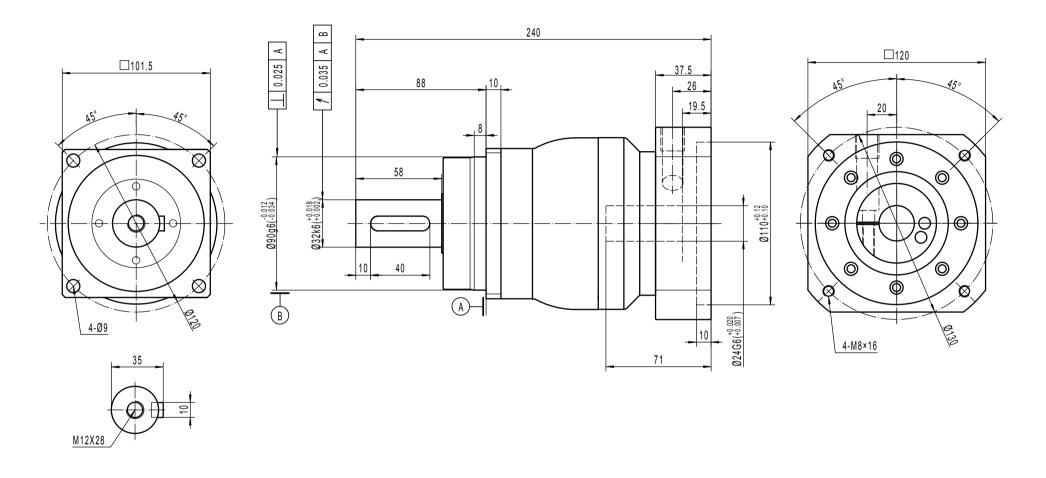
Note 1: This drawing shows the dimensions of X-Treme-SQ-ST-100 - 1 STAGE (this drawing is common to all ratios from 3 to 10)
