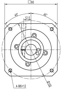
Note 1: This drawing shows the dimensions of X-Treme-SQ-ST-075 - 2 stages (It is common to all ratios from 12 to 100)
