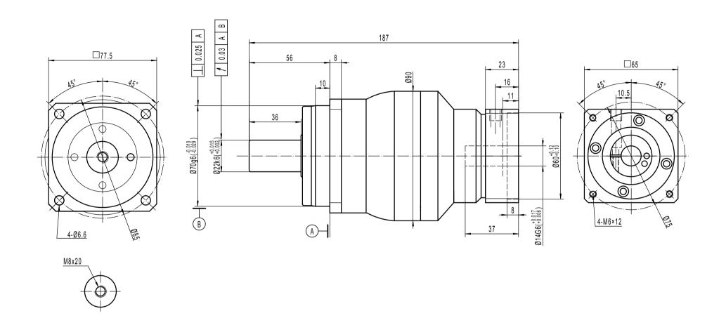
Note 1: This drawing shows the dimensions of X-Treme-SQ-ST-075 - 2 stages (It is common to all ratios from 12 to 100)
